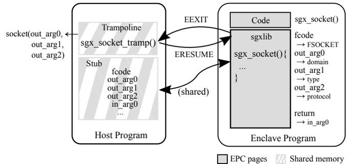
Fig. 4: Interface defined for communicating with the enclave’s host program that performs the delegated calls to the operating system. In this figure, a `sgxlib` library, `sgx_socket()`, running inside the enclave, requests a socket system call via *trampoline* and *stub*, which are pre-negotiated between the enclave and its wrapper when packaged together.
