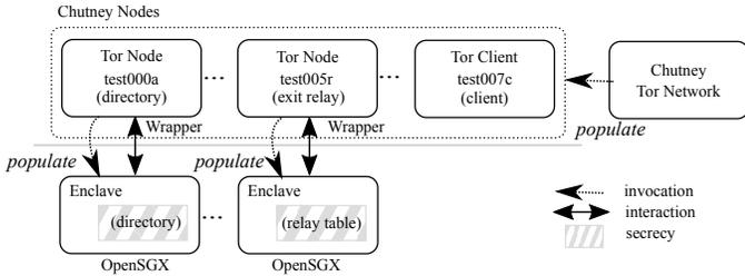
**Fig. 5:** An overview of the execution environment of an OpenSGX-enabled Tor. To reduce the size of TCB (an enclave program), we use SGX to protect the secrecy of Tor nodes; directory in Directory Node and relay table in Exit Node.
