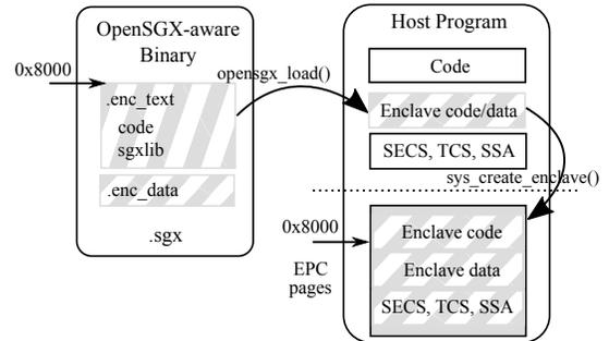
**Fig. 3:** Loading process performed by OpenSGX loader. First, `.enc_text` and `.enc_data` sections are loaded in to host memory. OpenSGX loader then forwards two sections along with stack, heap, and other necessary data structures to EPC via `sys_create_enclave()`.
