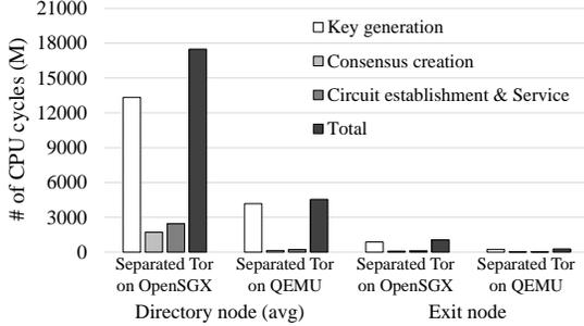
**Fig. 7:** The number of CPU cycles of Tor-enclave process for the three phases. Here, separated Tor on QEMU means executing Tor-enclave process without using SGX instructions and `sgxlib` calls on the native QEMU.
